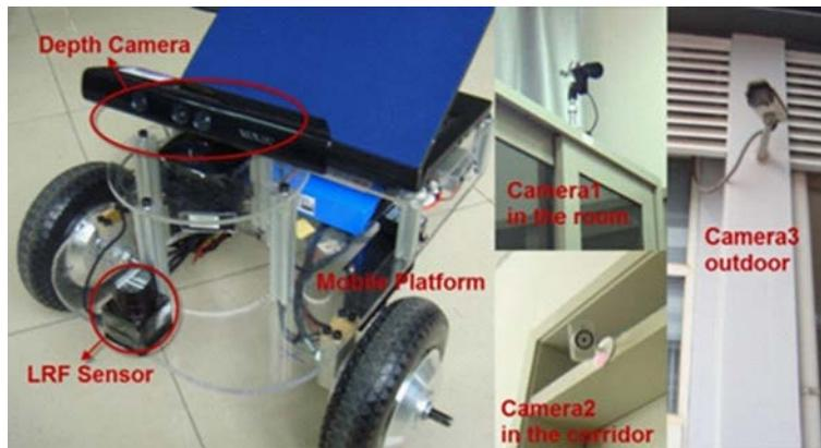
Figure 3 The environmental camera installation example
